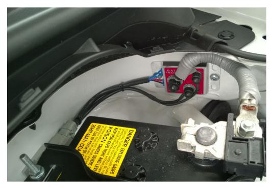
The Isolator should be mounted directly to the vehicle's metal chassis close to the vehicle's battery but away from any high temperature sources.
