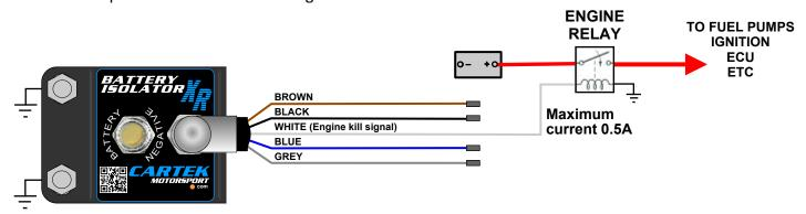
WARNING: The Battery Isolator must be fully connected before starting the engine. If the engine kill output signal is not connected when the engine is running then damage to the Battery Isolator may occur. (Cars without alternators do not apply).
