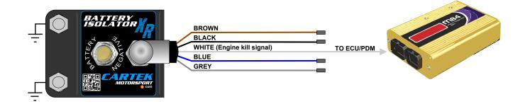
It is also possible to use the Engine Kill Signal to control an Engine Relay/DME. Please check the manufacturers specification before installing.
